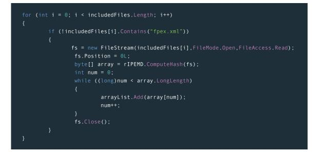
The usage of the Contains() method in: if (!includedFiles[i].Contains("fpex.xml")) facilitates the exploitation of this flaw.
