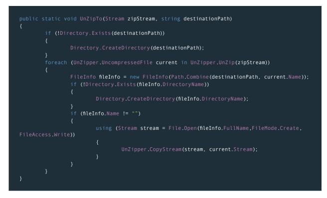
No checks are performed for the validity of filenames within the archive. As such, an attacker can craft a zip file with a filename that contains a relative path to traverse outside of the parent folder. For example, consider a zip archive containing a file with the following path:
